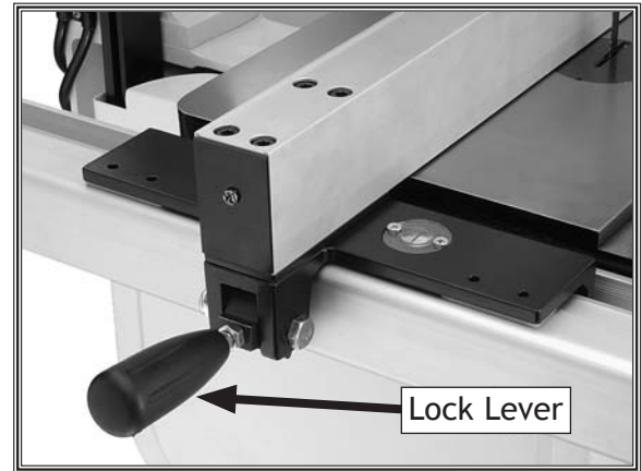
Figure 12. Fence secured in place.
